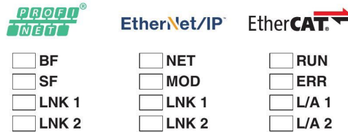
Figure 30 LED status indicators for PROFINET, EtherNet/IP™, EtherCAT®
